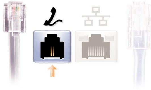
If your computer has an internal modem, connect the telephone cable to the modem connector and connect the other end of the cable to a telephone wall jack.
