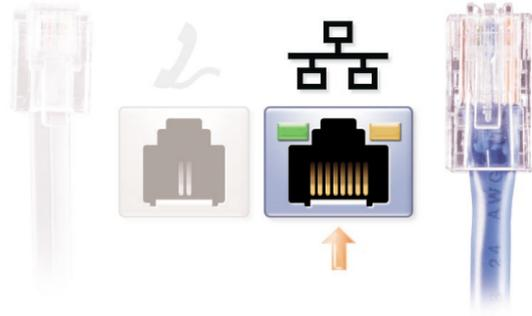
If your computer has a networking option, connect a separately purchased network cable to the network connector.
